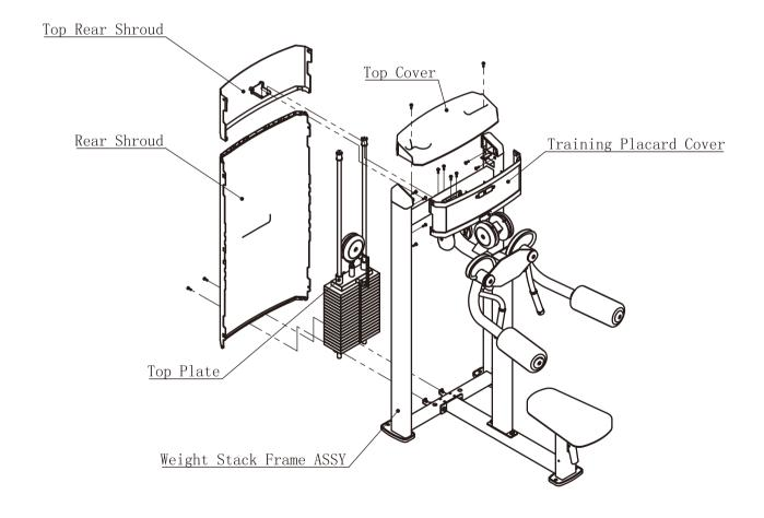
**STEP 2**Attach eight Plastic Nut (#6) to the Weight Stack Frame ASSY.
